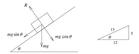
Resolving perp. to plane:  $R = mg \cos \theta$ Parallel to the plane (by Newton II)
